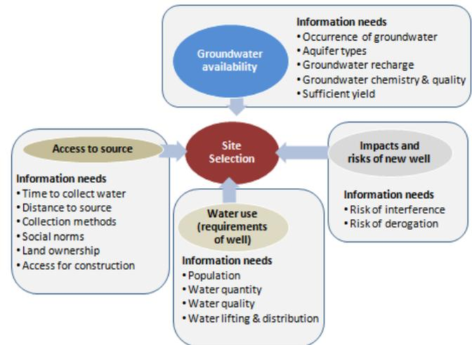
There are many techniques for well siting, each requiring different skills as well as investments in technology. These techniques are appropriate, either singly or in combination, for different geological and user settings. It is important that the appropriate techniques are utilised. Of particular mention is the fact that water-well siting in Africa tends to use geophysical surveys<sup>1</sup>, even though they are not always necessary.
