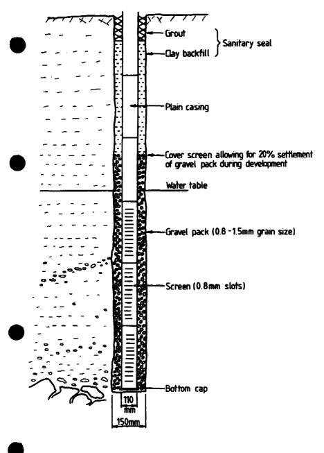
Simple Tube Well Design Fig T13/3
