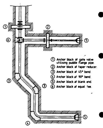
Typical Arrangement of Concrete Anchor Blocks used in conjunction with P.V.C. pipework incorporating rubber ring mechanical joints when buried. Fig T15 (
