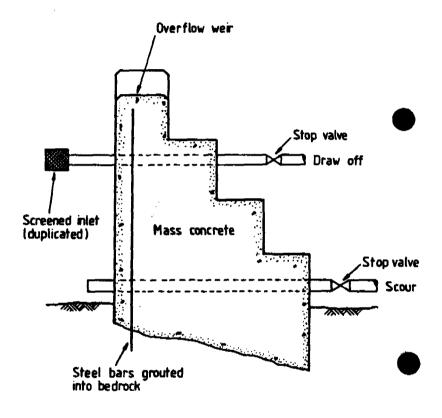
Small Gravity Dam Fig D7
