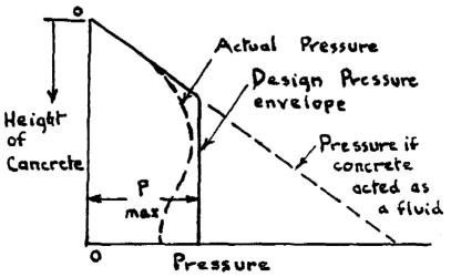
A full discussion of this subject is contained in CIRIA Report 108 (Concrete Pressure on Formwork) 1985, but for field use using normal Portland Cement concrete the approximate loading in Table 1 may suffice.
