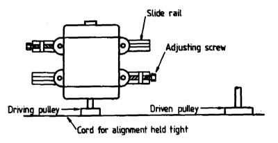
3. Alignment for Pulley Drive
