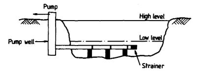
Note : Direct coupled pumps can be used if self-priming and suction head is not too great.
