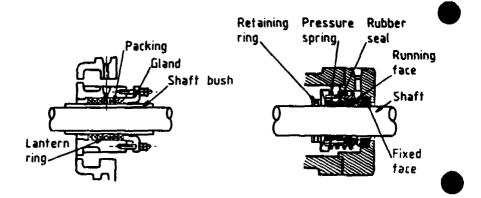
a) Soft-packed stuffing box b) Mechanical seal
