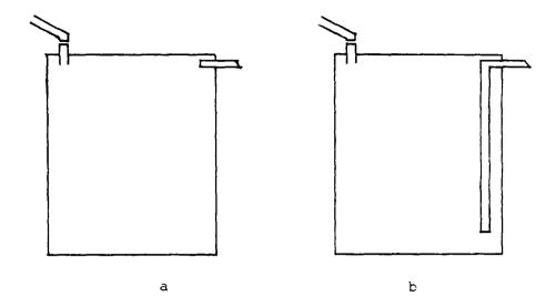
Figure 4.1 Design of Overflow Pipes for Tank Constructions.
