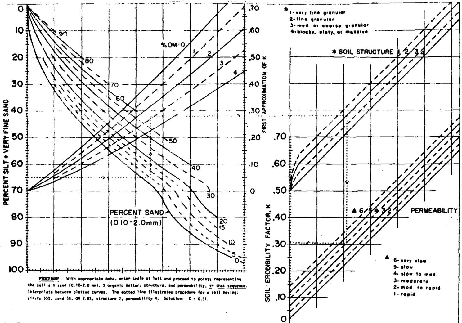
The soil-erodibility nomograph. Where the silt fraction does not exceed 70 percent, the equation is  $100 K = 2.1 M^{1.6} (10^{-3}) (12 - a) + 3.25 (b - 2) + 2.5 (c - 3)$  where  $M = (\text{percent si} + \text{vfs}) (100 - \text{percent c})$ ,  $a = \text{percent organic matter}$ ,  $b = \text{structure code}$ , and  $c = \text{profile permeability class}$ .
