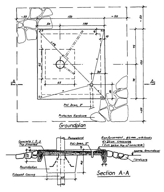
Material Needed for Platform (incl. Foundation):
