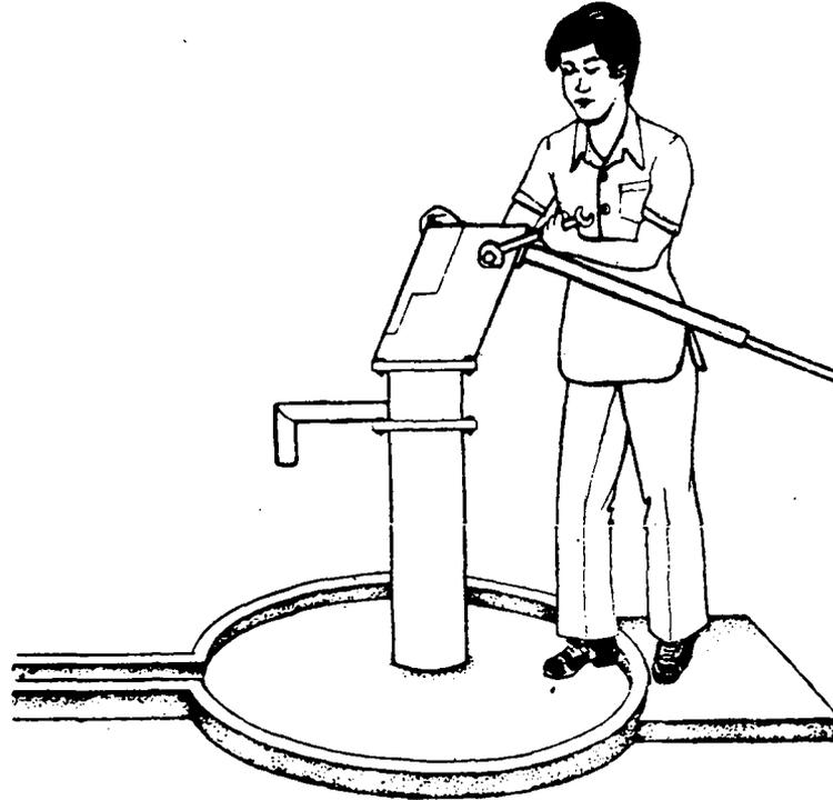
**1. Are axle bolt and lock-nut tight ?**
