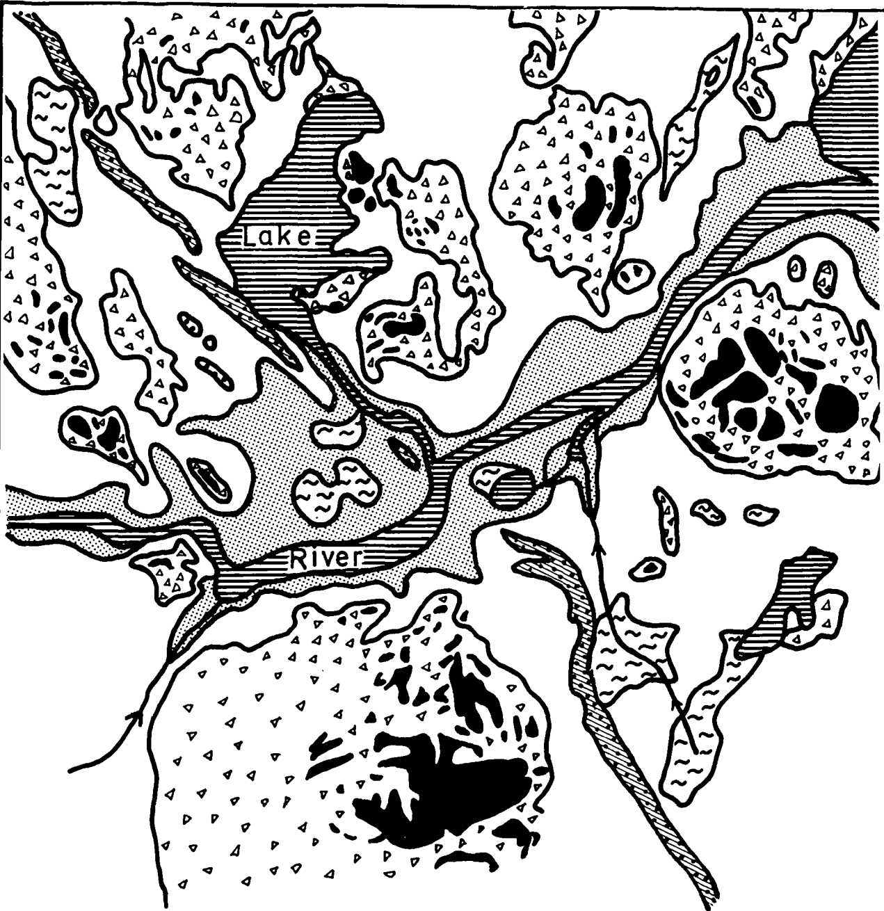
Fig.1. Common situation for an esker aquifer in central Sweden.
