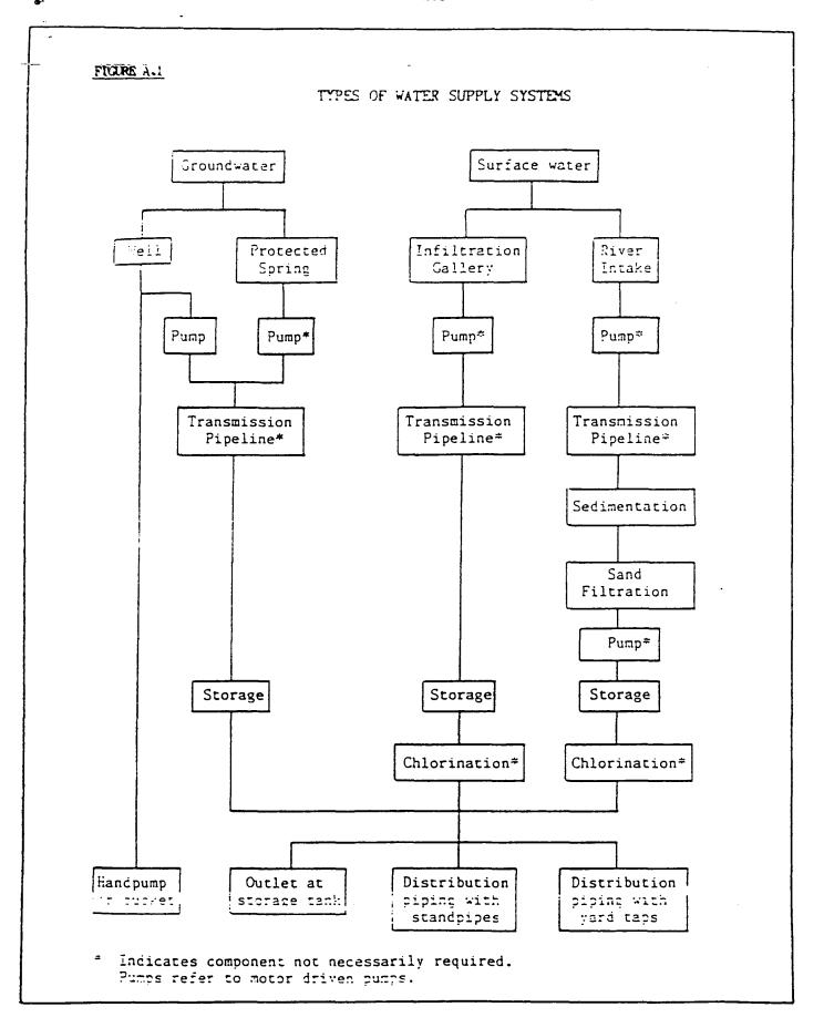
sand filter, water should pass through a settling tank prior to filtration. In addition, in order to meet World Health Organization bacteriological water quality guidelines (MPN of 3 coliform per 100 ml), surface waters must be disinfected (WHO, 1984). The need for continual attention to maintain such treatment processes and the requirement of an uninterrupted supply of chlorine result in almost inherent reliability problems with water treatment in rural communities.
