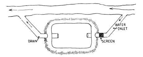
Diversion ponds can be made in a number of ways. Sometimes a pond is dug in flat ground or can be made by slightly enlarging a natural depression in the land.
