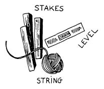
To survey the land for slope, some stakes (long, straight pieces of wood), some string (fishline, etc.), and a carpenter's level are needed.
