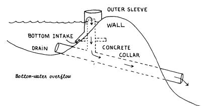
**DOUBLE SLEEVE OVERFLOW** This drainage system is built like the turn-down pipe, except a large pipe is placed over the section of pipe which extends above the pond's surface. This outer pipe should be longer and wider than the inner pipe, which is placed so that it is about equal in height to the depth of water desired in the pond.
