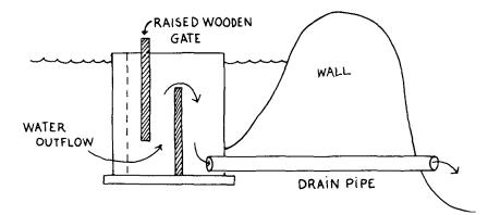
There are other ways this kind of monk can be built. For example, the second groove could be filled by a large wooden gate (one piece of wood or several fastened together) which could be raised and held up to allow a flow of water from the bottom of the pond. It is this flow of water from the bottom of the pond which is important.
