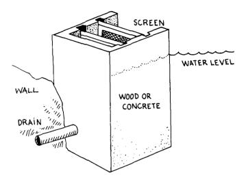
A monk-type drainage system controls the level of water and prevents fish from escaping when the pond is being filled. It also allows for good drainage of the pond. The completed structure consists of a horizontal drainage pipe and the vertical structure, or monk. The drainage pipe must be placed before the walls are built; the monk may be built outside the pond, and placed inside later.
