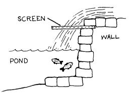
The horizontal screen at the left is very effective. Here the screen is placed so that the water passes through as it falls into the pond. This screen merely juts out from the wall at the inlet.
