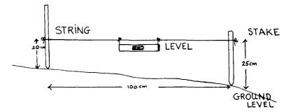
This drawing shows that one string is tied at 20cm; the other is tied at 25cm. Therefore, one end of the area is 5cm lower than the other. The distance covered by the string is 100cm, so the slope is 5% (over 100cm of ground, the elevation changed 5cm). Since a slope of 2-5% is good for a fish pond, this site has a satisfactory slope for a pond.
