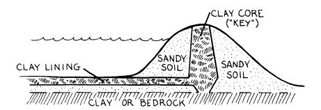
If the farmer has a soil which is a mixture of clay and sand, and he is not sure it is strong enough, he may still wish to build a clay key. Or he can build a key using the same soil used in the wall. This key must be packed down very tightly.
