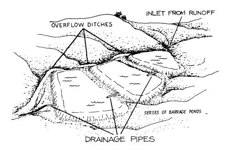
The number of pond walls the farmer must construct depends upon the land and on how he fixes his drainage system. A barrage pond usually needs only one wall -- the main wall between the water source and the pond area. One kind of drainage system called a sluice (see "Construction" section) can be used to let water both in and out of the pond. There are also a number of simple drainage systems which can be used that do not require any complicated construction.
