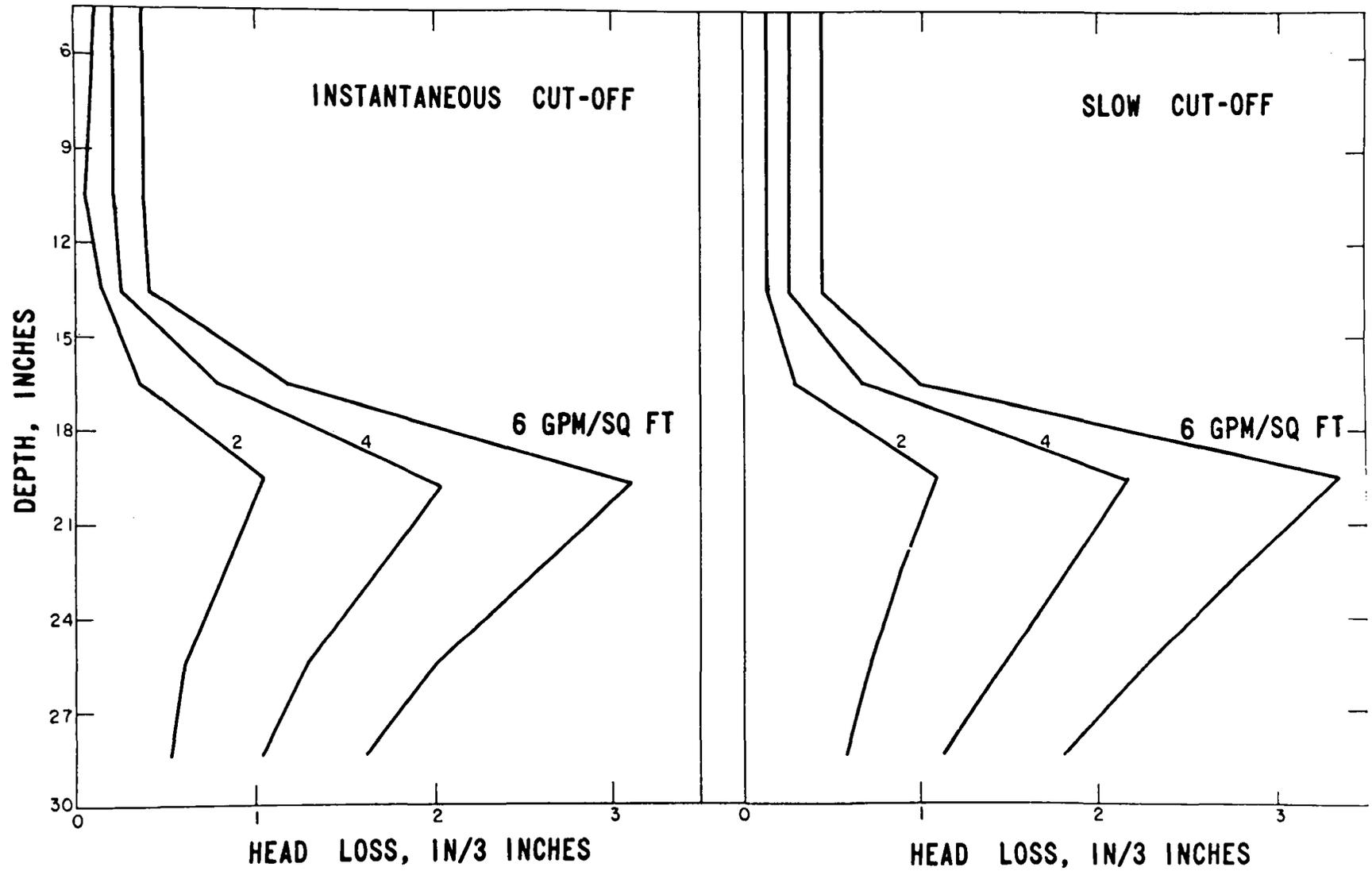
FIGURE 16. Head Loss Gradient, Dual Media.
