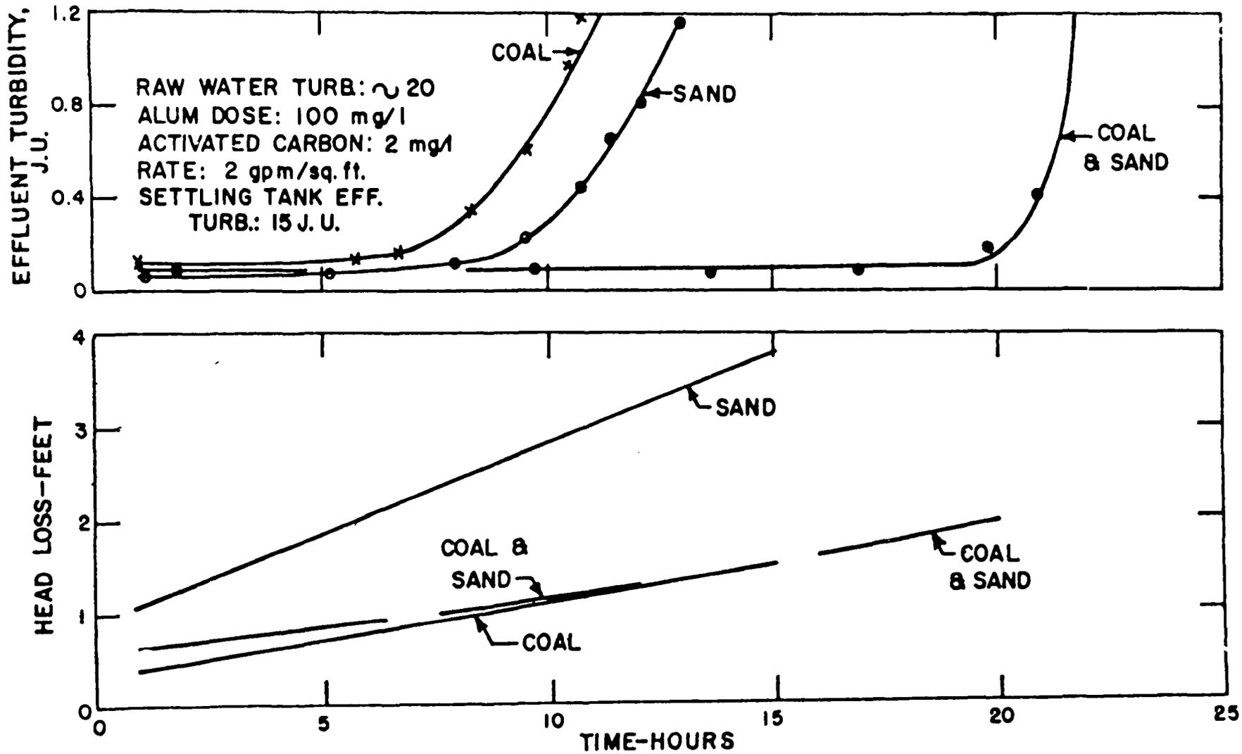
FIGURE 3. Influence of Filter Media on Length of Run with Weak Floc.
