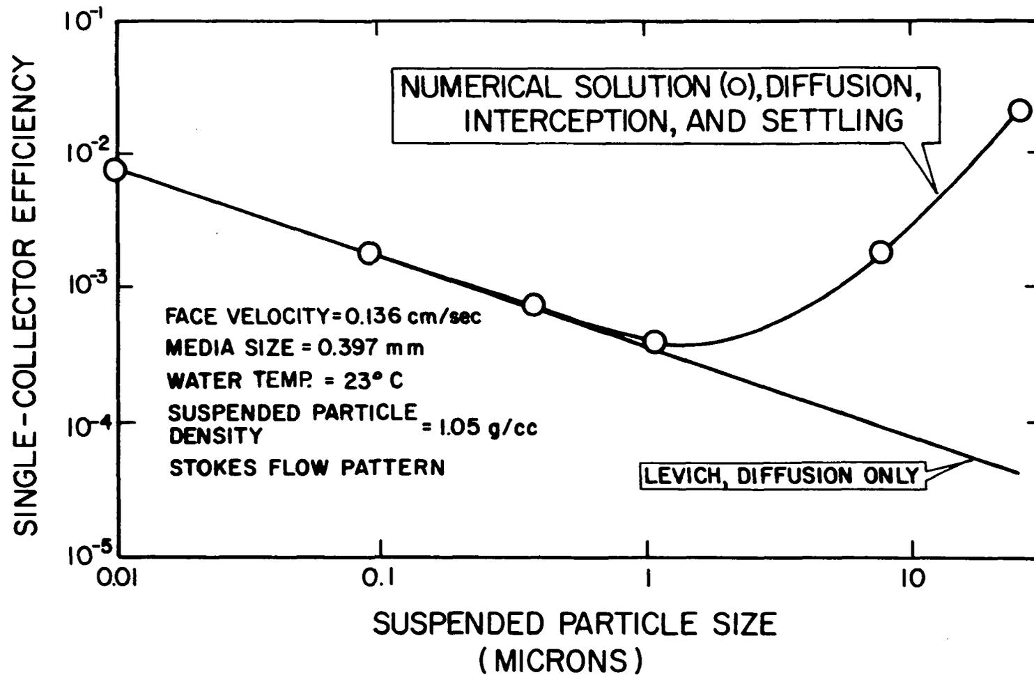
FIG. 4 THEORETICAL PARTICLE TRANSPORT EFFICIENCY IN A POROUS MEDIUM (YAO AND O'MELIA [4])
