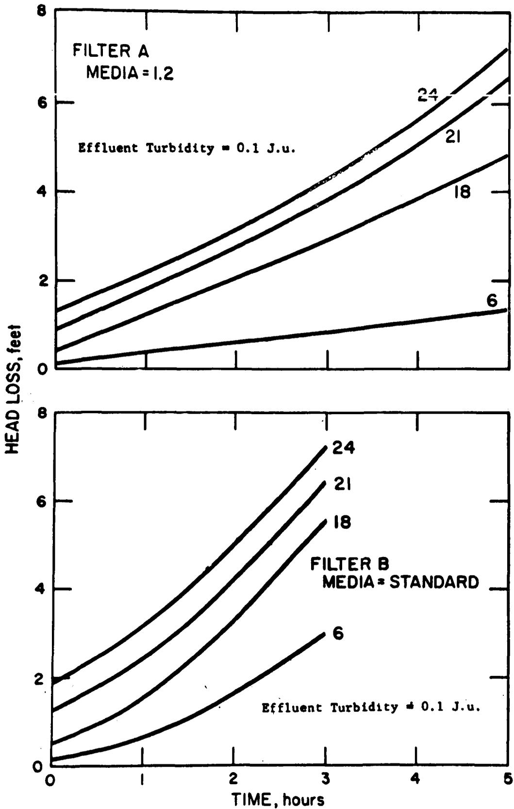
FIGURE 12. Influence of Filter Media on Run Length (6 gpm/sq ft, 10 mg/l Alum, Influent Turbidity 35 J.u.).
