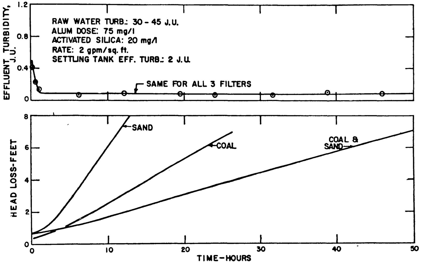
FIGURE 4. Influence of Filter Media on Length of Run with Strong Floc.
