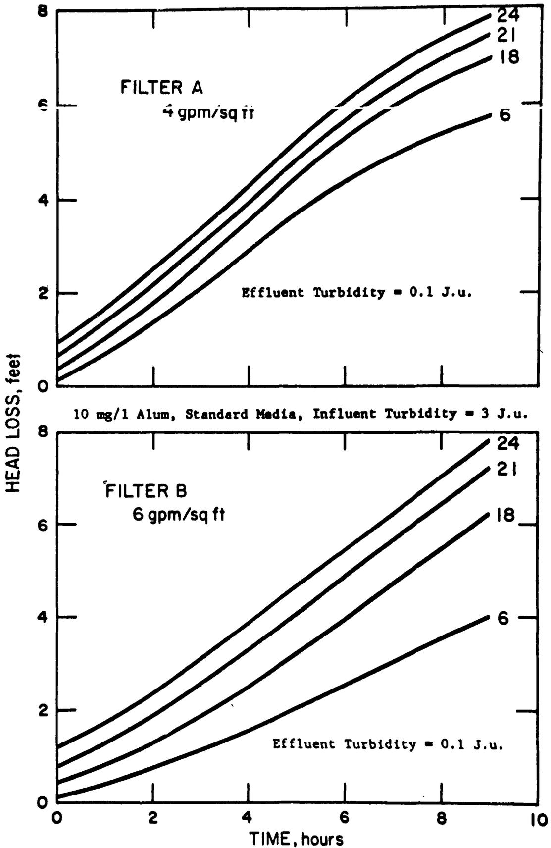
FIGURE 10. Influence of Filtration Rate on Run Length.
