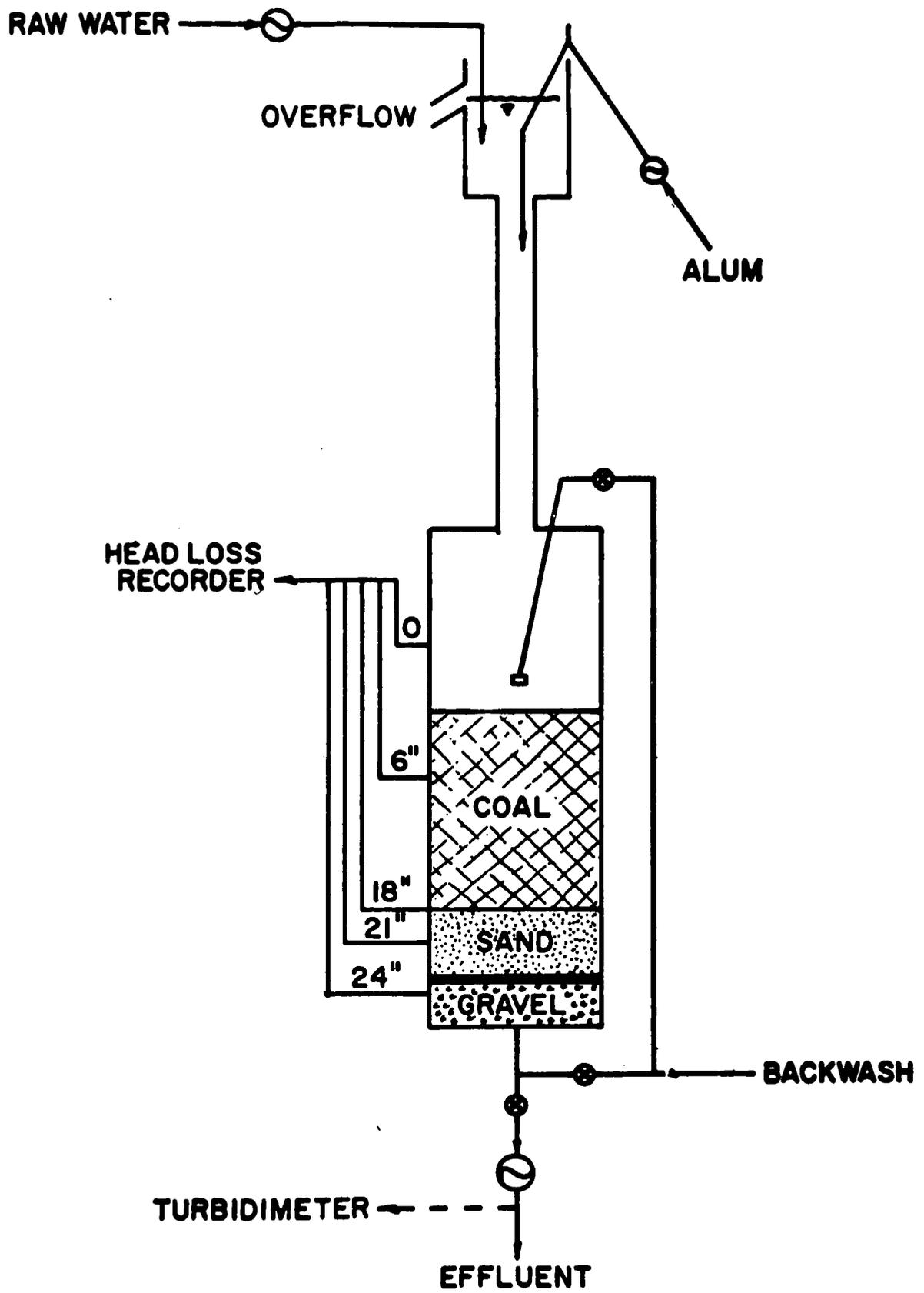
FIGURE 1. Details of Experimental Filter.
