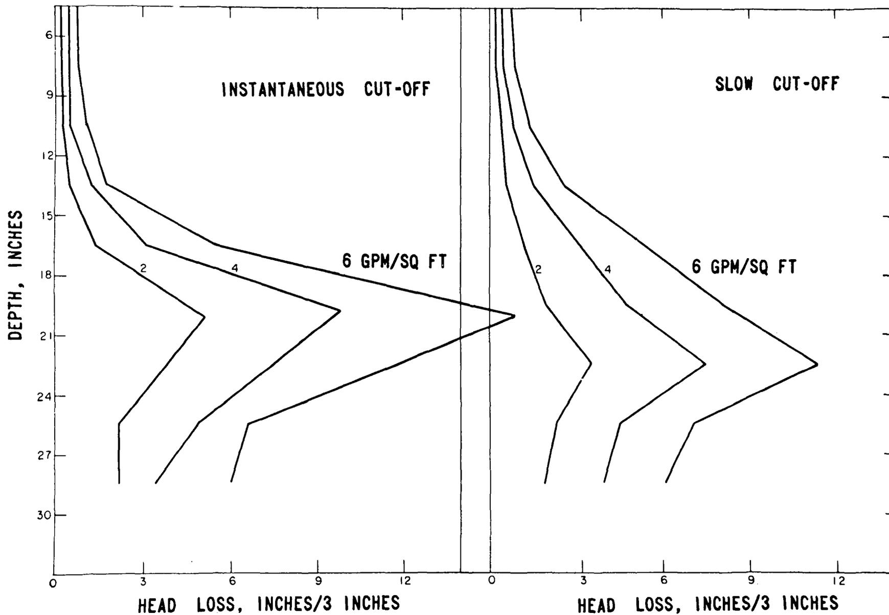
FIGURE 19. Head Loss Gradient, Dual Media Special.
