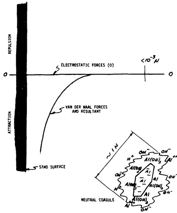
shape of the clay and the fact that some clays (kaolinite for example) may have both positive and negative regions at low pH, it is not unexpected that some penetration of the barrier will occur and some of the particles will be separated from suspension. Note especially the small range of the barrier compared with the size of the particle.
