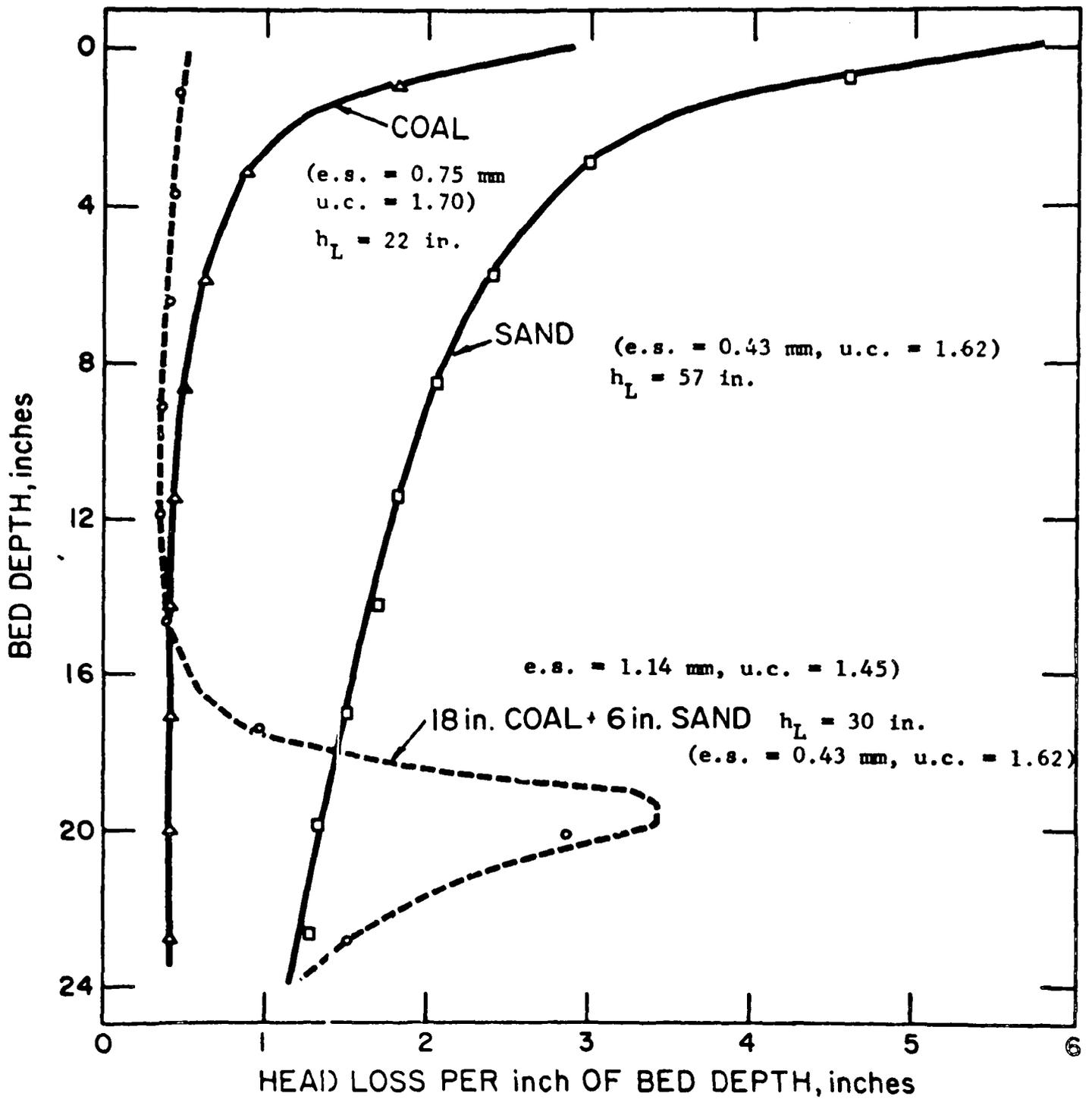
FIGURE 15. Clean Water Head Loss for Three Filter Media at 14.5 gpm/sq ft.
