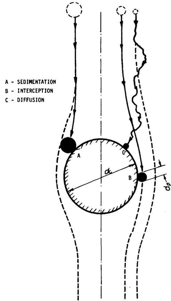
FIG 3. TRANSPORT MECHANISMS
