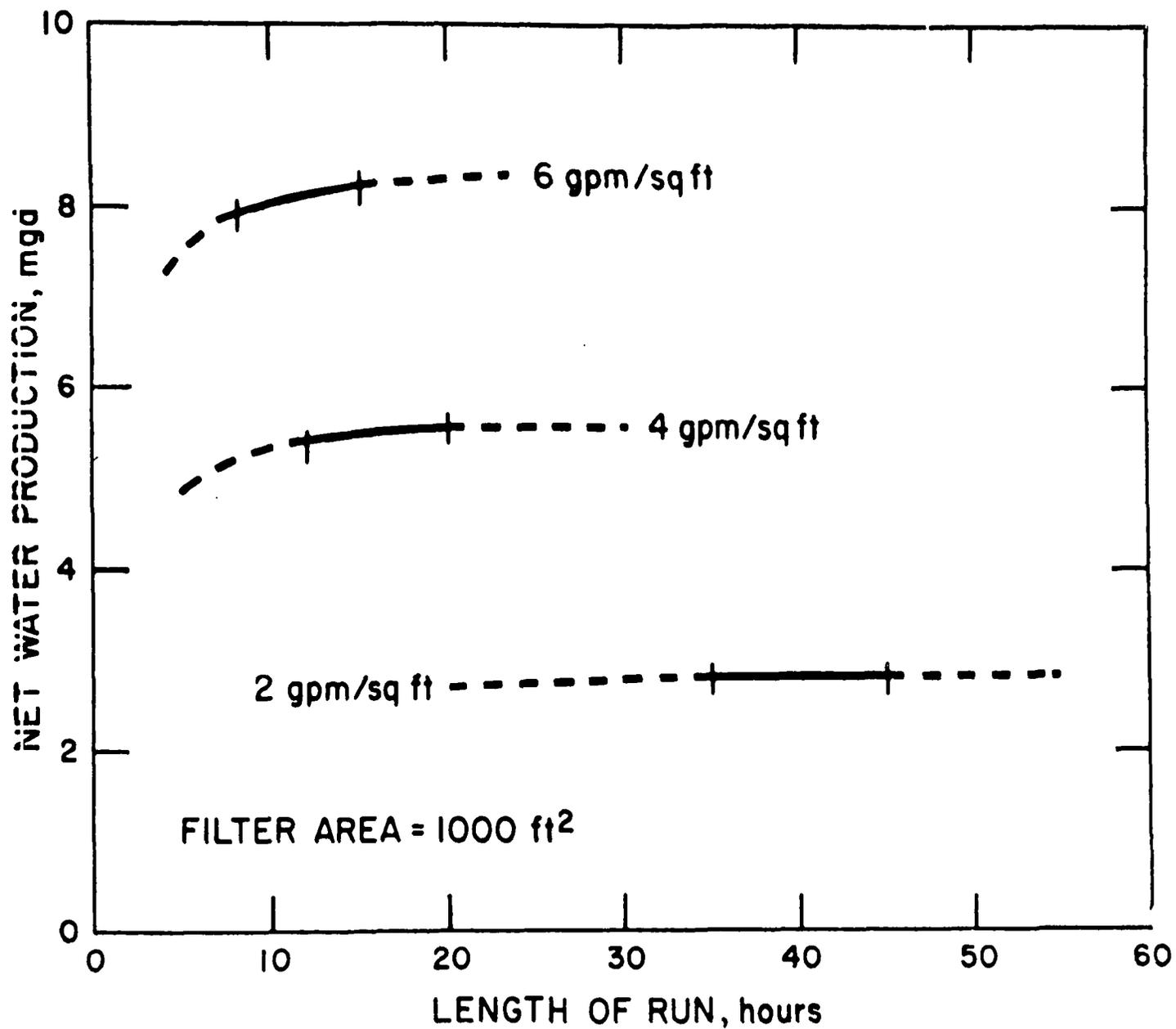
FIGURE 11. Influence of Filtration Rate and Run Length on Net Water Production.
