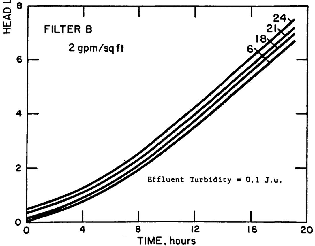
FIGURE 9. Influence of Filtration Rate on Run Length.
