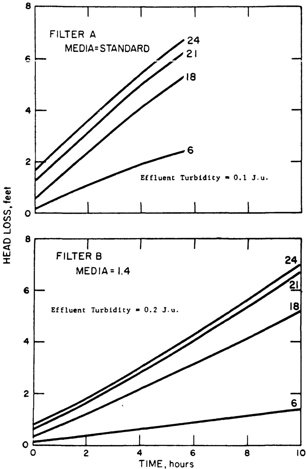
FIGURE 13. Influence of Filter Media on Run Length (4 gpm/sq ft, 10 mg/l Alum, Influent Turbidity=7 J.u.).
