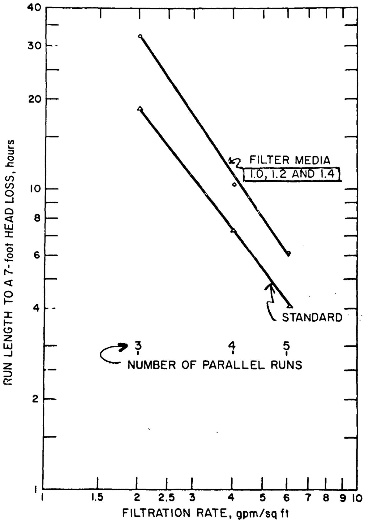
FIGURE 14. Influence of Filtration Rate and Filter Media on Run Length.
