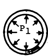
Fig. 14: Pipe exposed to internal hydraulic overpressure.
