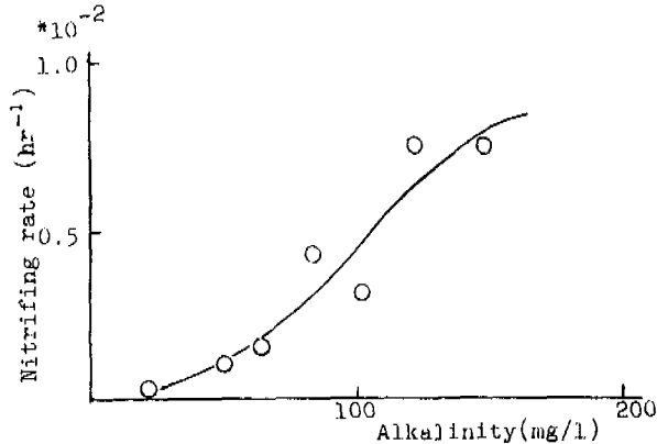
Fig.2 The effect of alkalinity on the nitrification rate
