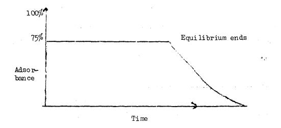
The removal by activated aluminium oxide of organic substances such as chlorine, lignin and sulphuric acids, from the bleaching process in pulp and paper industry has been investigated at a small scale. Regeneration of aluminium oxide is achieved by heating to about 700°C. Further research is in progress to improve the cost effectiveness of the process and to apply aluminium oxide as an adsorbant for recovery of phosphates.
