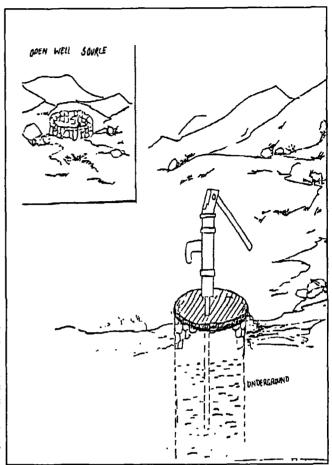
The lining under the water level, prevents the well from collapsing and facilitates groundwater entering the
