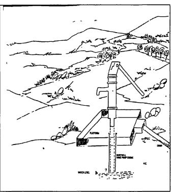
The pump rods have special connectors allowing for assembly and dismantling with no or only very simple tools. The joints incorporate pump rod centralizers that prevent water of the rising main. To a large extent improved models can be maintained at village level. Such type of hand pumps are India Mark III hand pumps.
