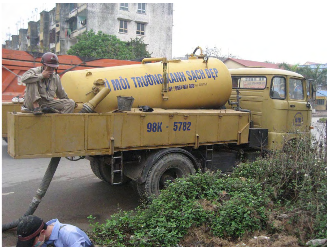
A private desludging company empties the contents of its vacuum truck into a city drain. In Vietnam, where most cities rely on both public and private providers, private participation poses both a challenge for regulators, and an opportunity to expand and improve desludging services.
