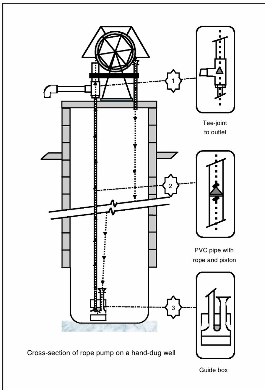
Figure 1 Cross section of a rope pump on a hand-dug well
