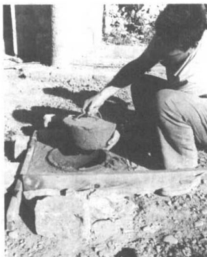
Figure 4. A concrete plug being placed in the test cover-slab.
