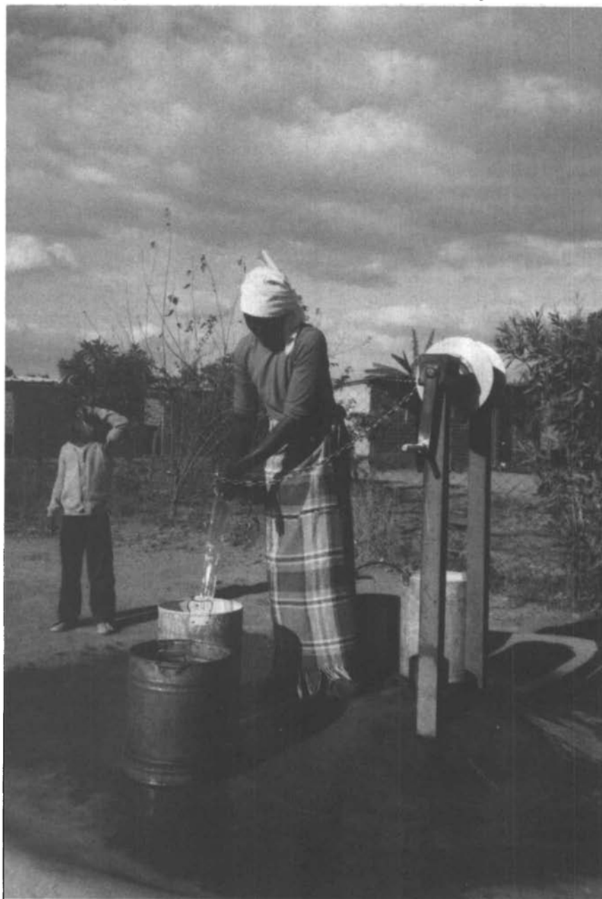
Bucket Pumps are simpler and are usually maintainable by the users.
