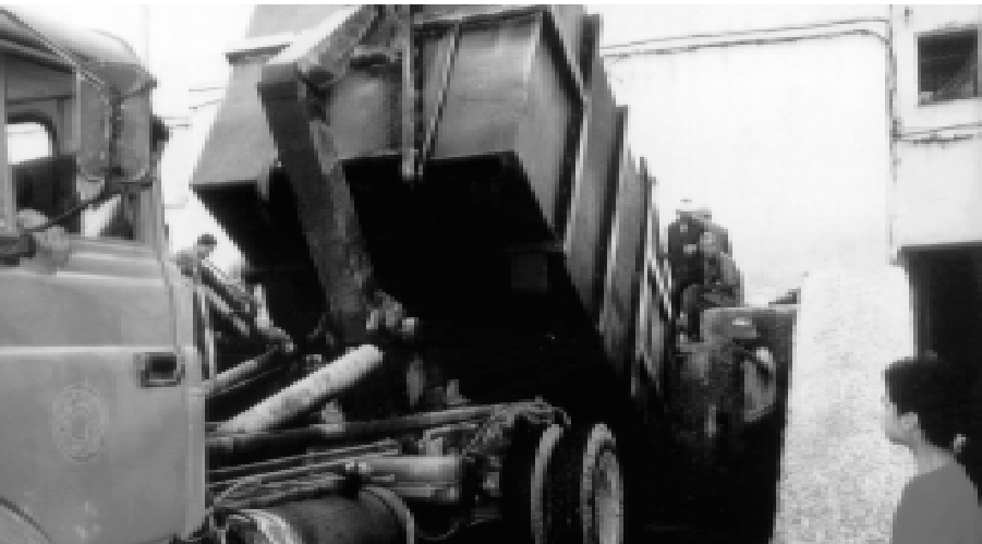
Photograph 3.2 An arm roll truck picking up a container in the Medina district of Fez (Morocco), 1985. (Waste had been brought to the container by a contractor using donkeys because of the access problems in the narrow lanes.)
