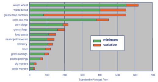
Figure 2.2. Typical gas yields of different feedstocks (after Austin, 2011)
