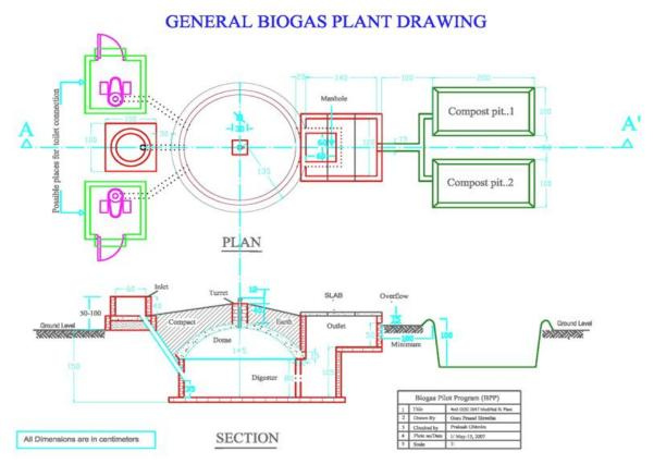
Figure 4.1. General biogas plant drawing for the Sinidu model GGC 2047
