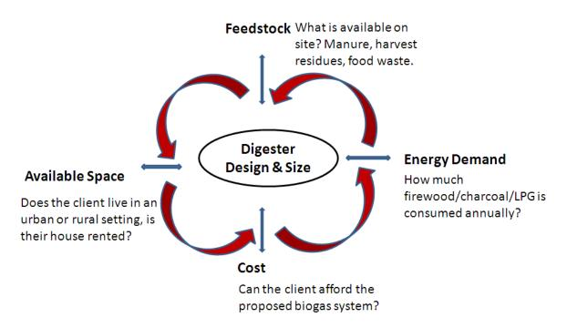
Figure 2.5. Factors that determine the optimum design and size of biogas digester. (Tumwesige & Casson, pers.comm. 2011)
