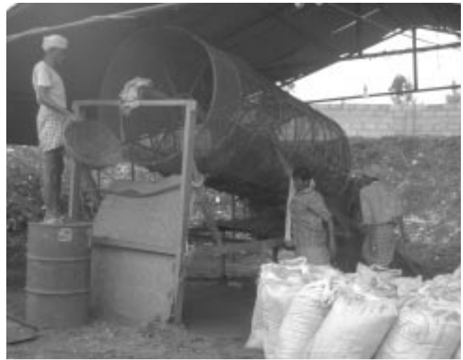
Photo 8. Trommel screen in use in Bangalore, India Photo: ©WASTE, Esha Shah
