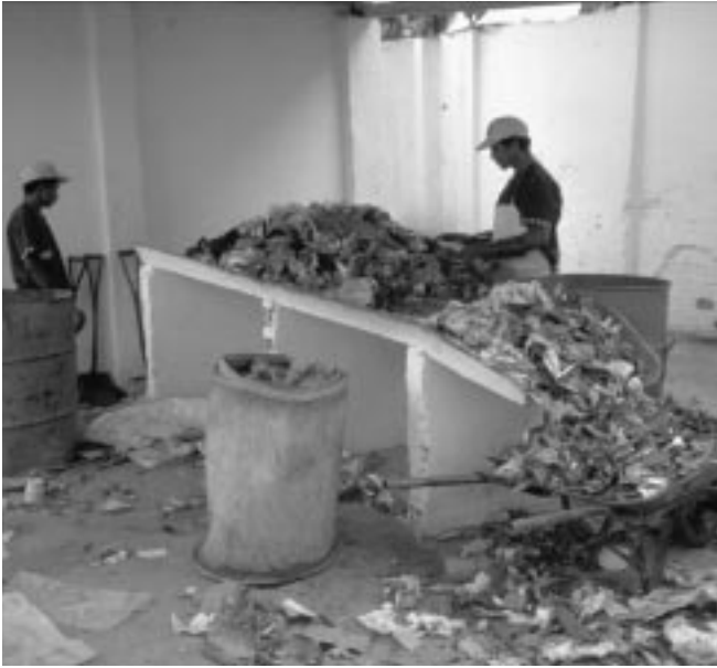
Photo 4. Workers are sorting out non-organic waste at compost site, Brazil
