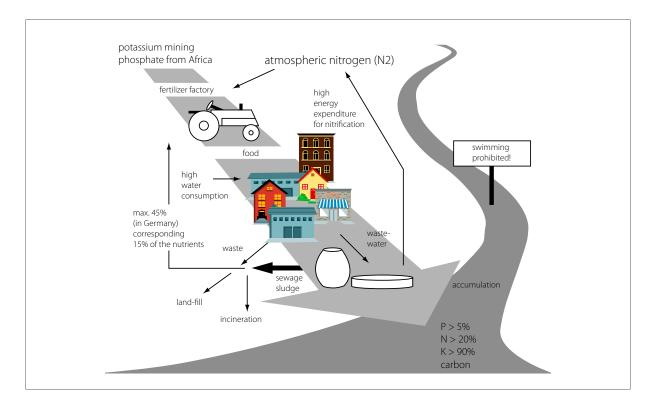
Figure 1: Material flows in the conventional sanitary concept (Source: Otterpohl et al., 1997)
