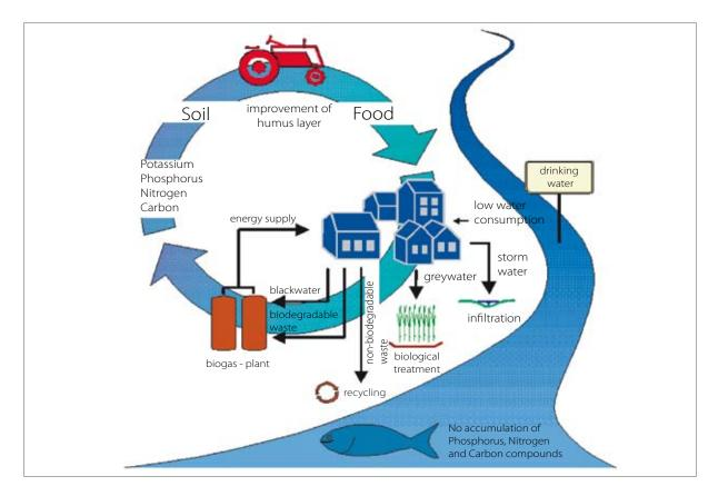
Figure 3: Material flows in ecological sanitation (Source: Otterpohl et al., 1997)
