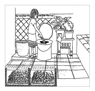
Composting toilet needs 0.2 l per flush, only for cleaning the toilet seat. There are also urine diversion composting or dehydration toilets (Figure 6 and 4 right). These lowflush and non-flush toilets save not only water, but also produce low diluted or dry faecal material that is easier to manage than highly diluted faecal wastewater as in conventional systems.
