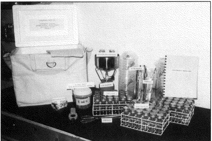
The portable water quality testing kit provides all the necessary equipment to test for bacteriological contamination of water sources in remote areas.
