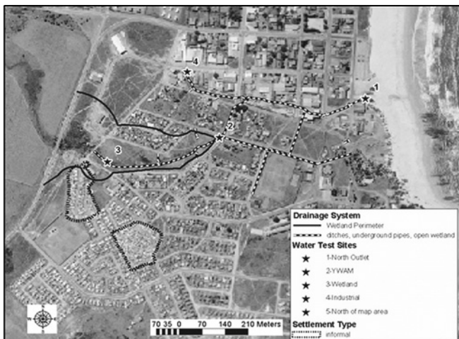
Aerial photos incorporating GIS map with a) wetland indicated by solid line, and ditches and underground pipes shown by dotted line; and b) a closer view with white areas representing concentrations of solid waste
