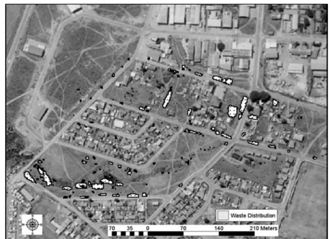
Aerial photos incorporating GIS map with a) wetland indicated by solid line, and ditches and underground pipes shown by dotted line; and b) a closer view with white areas representing concentrations of solid waste
