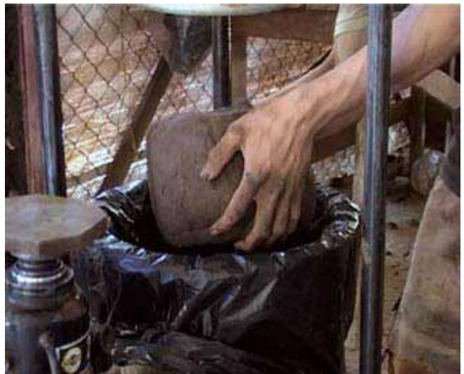
...and put into a mould with a plastic sheet layer to prevent the clay from sticking.
