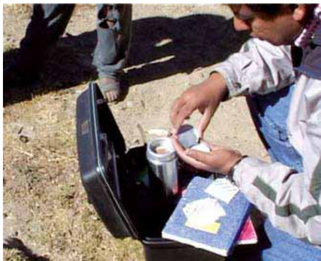
SODIS staff perform water tests regularly with this mobile laboratory, showing results some 14 hours later.
