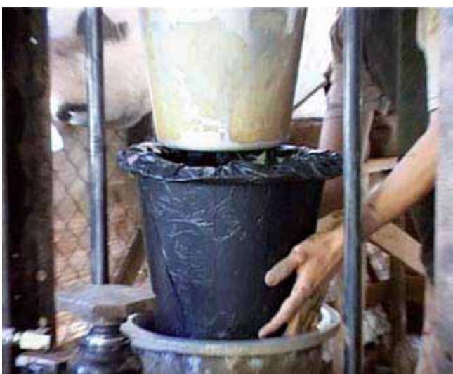
The filter is formed in a hydraulic press and the inner form is released
