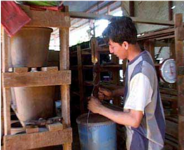
Production in Central America: it starts with measuring clay and sawdust
