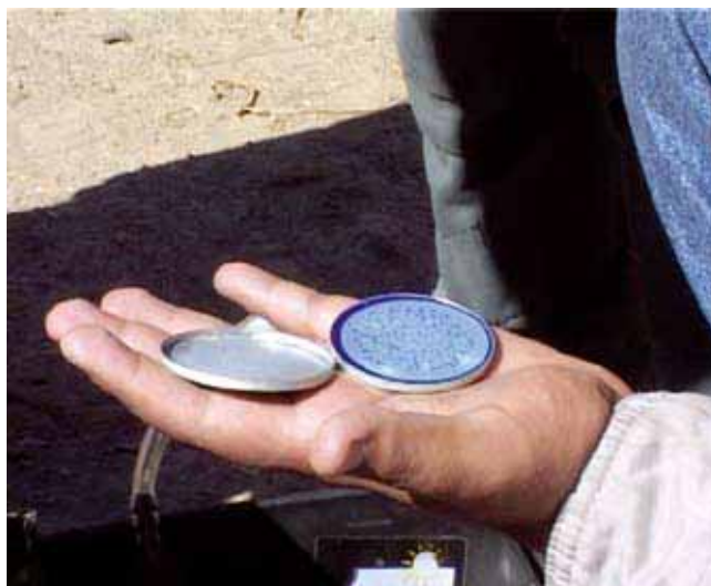
If the water is contaminated, dark spots develop in these petri dishes. It is not always easy for local people to understand these tests.
