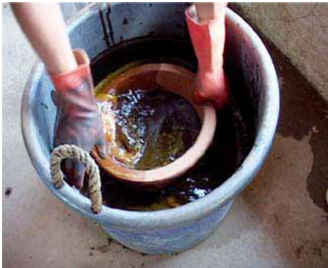
The filters are treated for 45 seconds in a bath with colloidal silver
