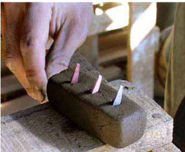
If two cones melt and the last one does not, then the fire has reached the required 900°C
