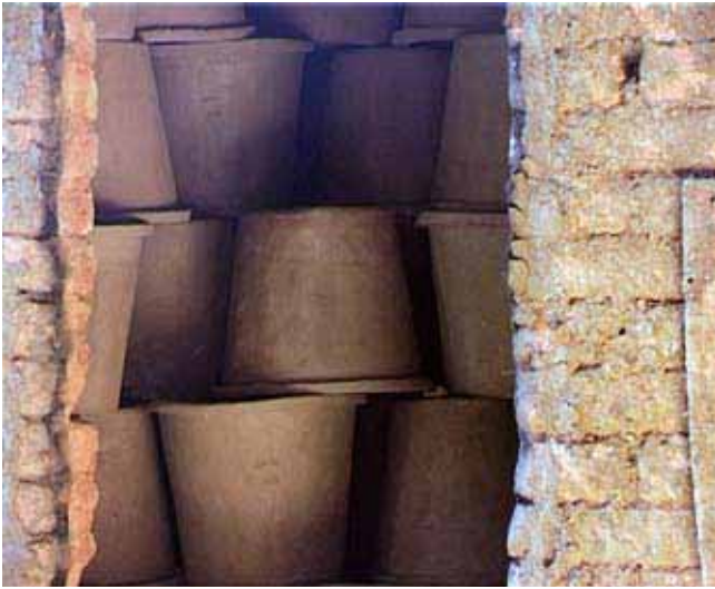
The filters are then stacked meticulously in the firing kiln
