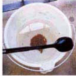
Floc formation after complete stirring
