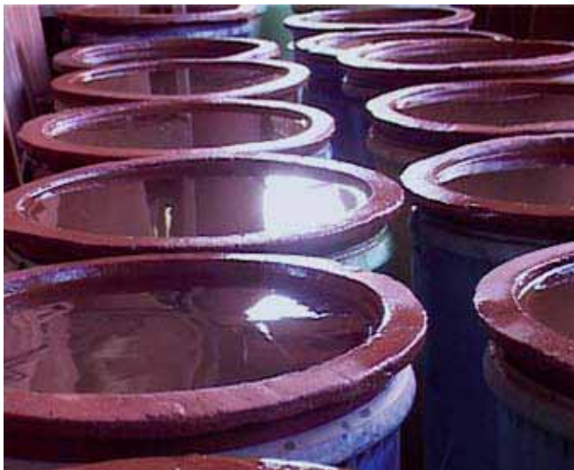
All filters are tested for quality: they are filled with water for one hour...
