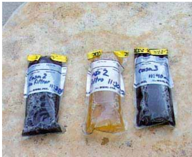
The first sample (left) is unfiltered water from the well at house Number 2. The second sample (centre) is from that house's filter. The yellowish colour indicates that the filter is protecting properly. The sample from house 3 shows re-contamination of the filter. The HACH test only indicates the absence or presence of bacteria, not how many are present.
