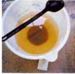
Floc formation after PUR addition
