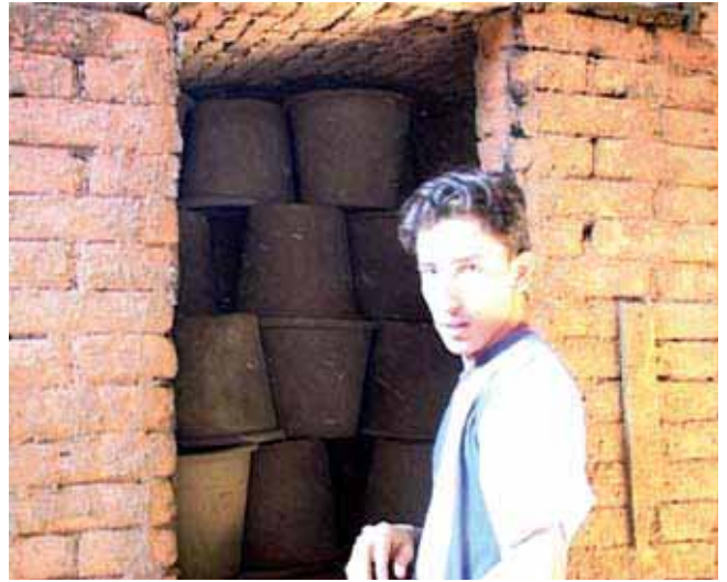
Some 50 filters can be fired in one batch in this firing kiln.
