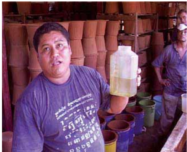
...and pass the test if the filtration rate is more than one and less than 2.5 litres
