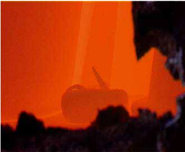
A view through the firing hole into the kiln. Only one cone has not yet melted.
