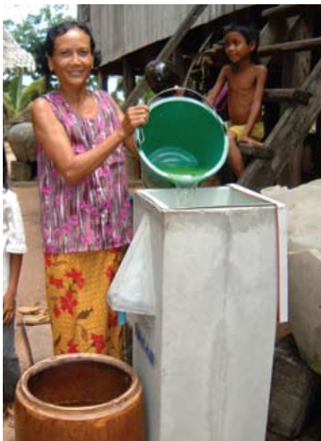
Filling the Biosand Filter
