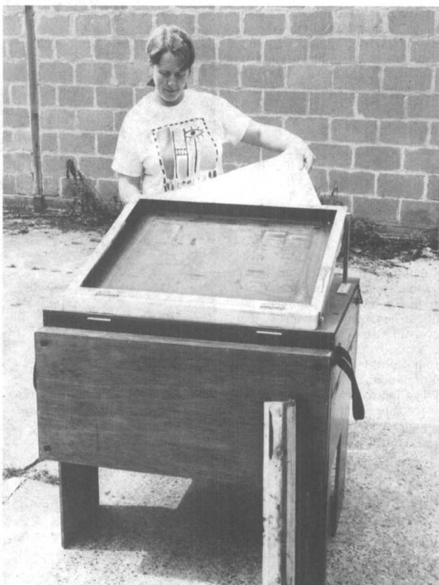
Demonstrating a portable silk screening unit that needs neither piped water nor electricity.
