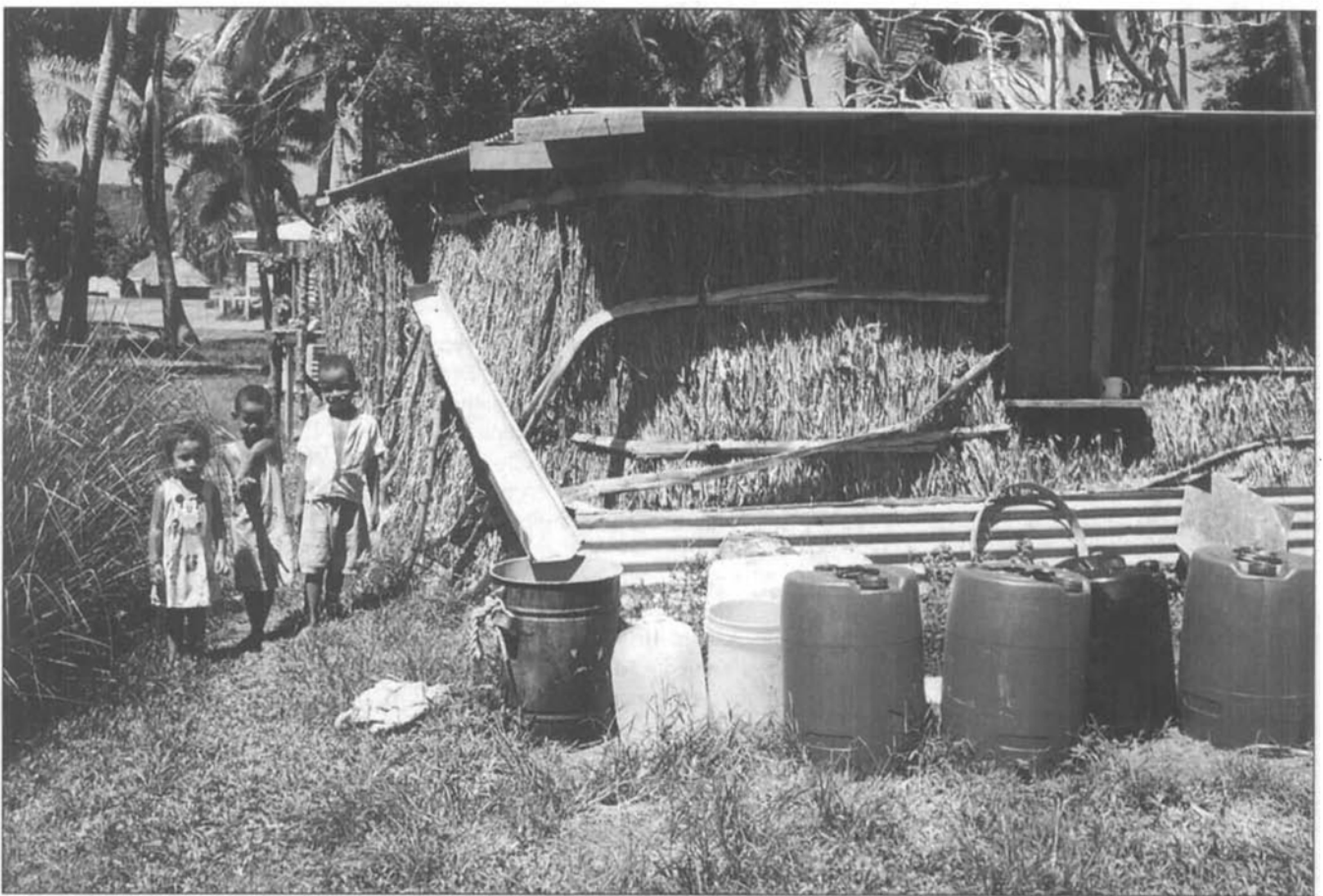
The most common rainwater catchment system — a gutter, a bucket, and several containers for storage.
