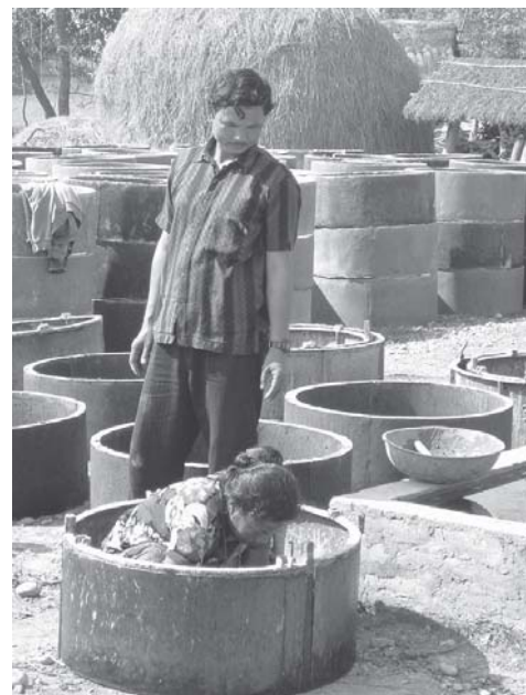
Latrine rings under production
