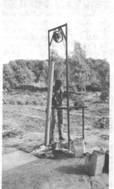
This 2m-long bailer and winch can lift 18 litres at a time, or 40 litres per minute.
