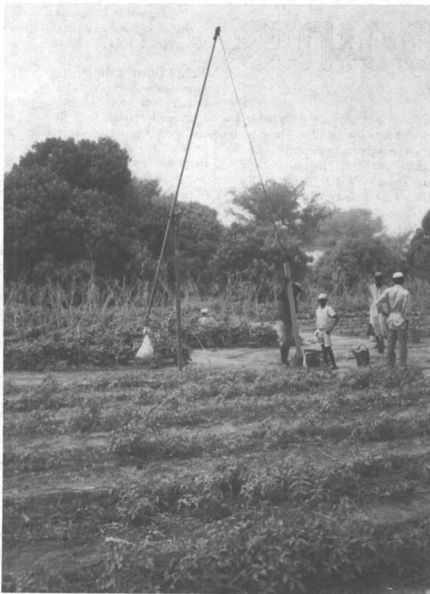
The hand-augered well coupled with a 3000-year-old technology, the shadaif, results in a hybrid system that can raise about 60 litres per minute.
