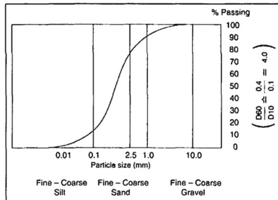
Figure 2. Sketch of particle size distribution.
