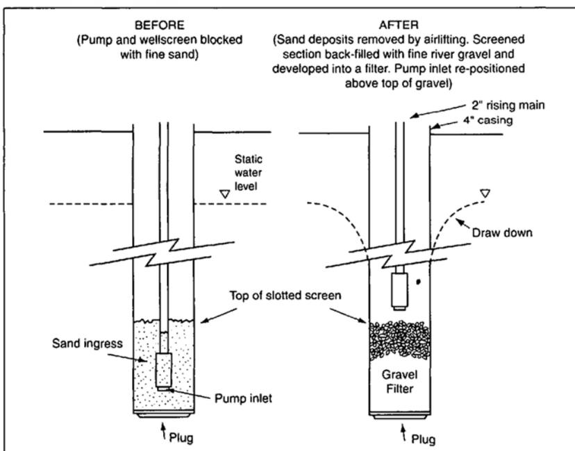
Figure 1. Borehole rehabilitation schematic.
