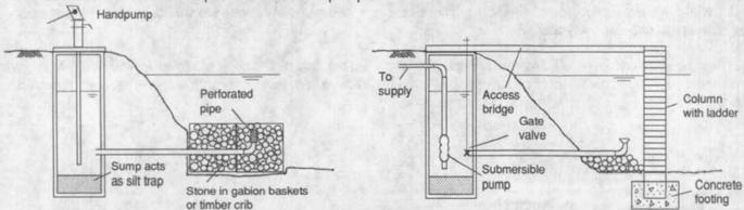
Problems can arise with all of the above intakes if the river bed is unstable (for example, gravel), or the river is very shallow at low flows. It can be difficult to set the intake level to be safe from silting up during floods, but still able to abstract water at low flows. A weir can assist with this (see opposite) or a floating intake can be used.
