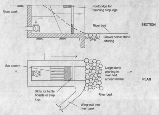
In the side intake the water is abstracted through an intake built in the river bank. The example includes wing walls into the bank and large stone pitching to protect the intake against floods and scour. A duplicate intake may be provided to facilitate maintenance.
