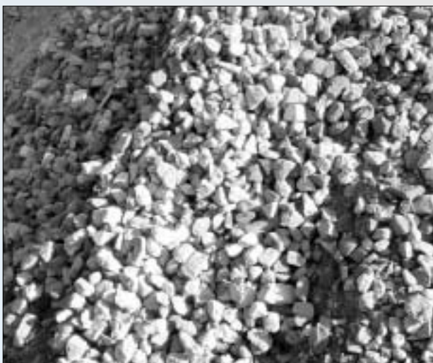
Clean, sized aggregate processed from building demolition waste at the POWSUS plant in the Netherlands
