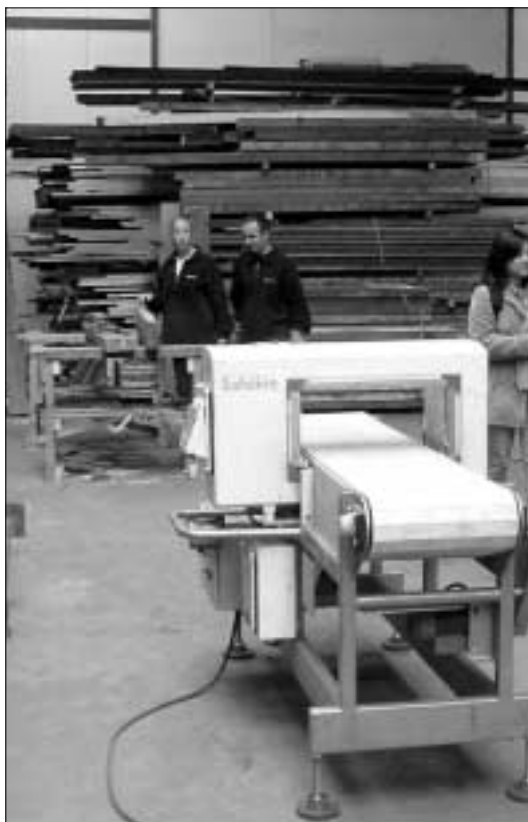
At a Dutch company specializing in recovery of old building materials for reuse, nails are removed from planks, which are checked in a metal scanner (foreground) and remilled
