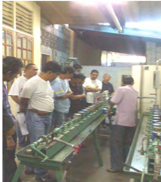
Engr Romulo Diaz (man in pink shirt, back to camera) of LWUA shows the JMWD trainees how to calibrate water meters.
