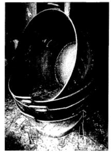
**Figure 3.9. Buckets, Tubes and Stools are Made of Tyre Sidewalls, Indonesia.** *Source: WASTE*.
