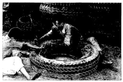
**Figure 3.10. Manual Separation of the Tread from the Sidewalls, Karachi, Pakistan.** *Source: PCSIR*
