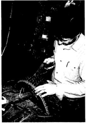
**Figure 3.3. Following the Grooves is a Labour Intensive Process.** *Source: Knud Sauer*.
