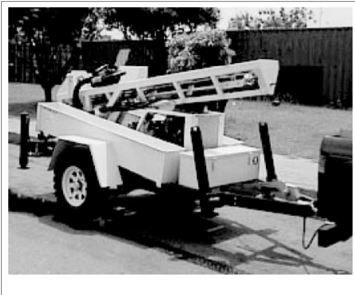
Figure 11: Rig in transporting position.
