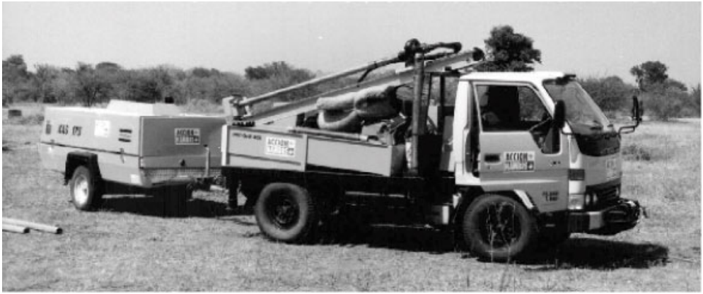
Figure 8: ACF-PAT 401. Rig on a Dyna truck.
