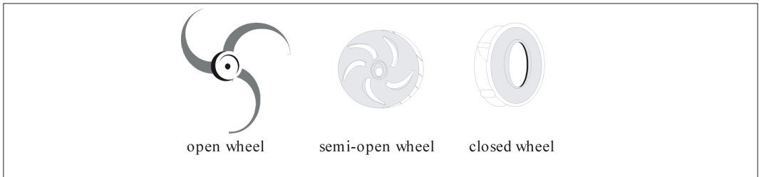
Figure 9.3: Rotor designs in centrifugal pumps.
