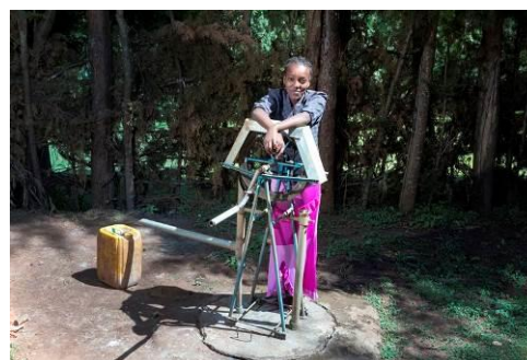
Photograph 2. Rope pumps are being promoted to upgrade family wells
