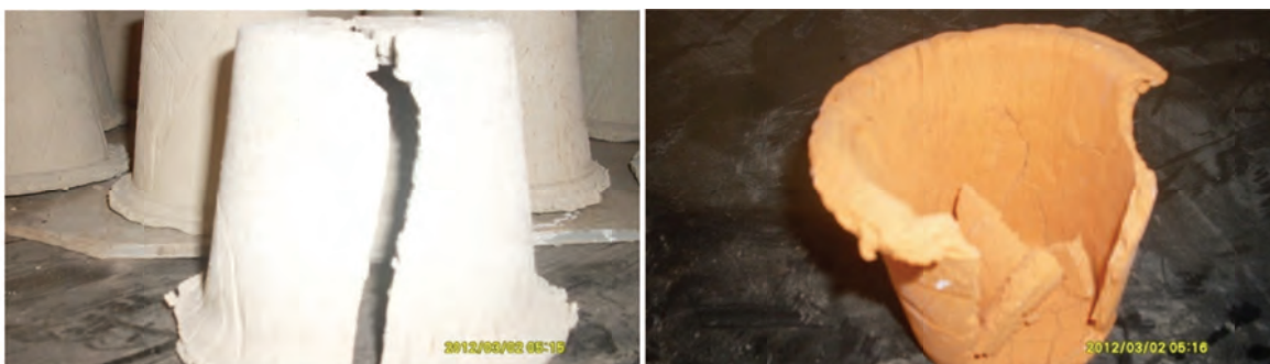
Figure 27: Cracks due to physical stresses
