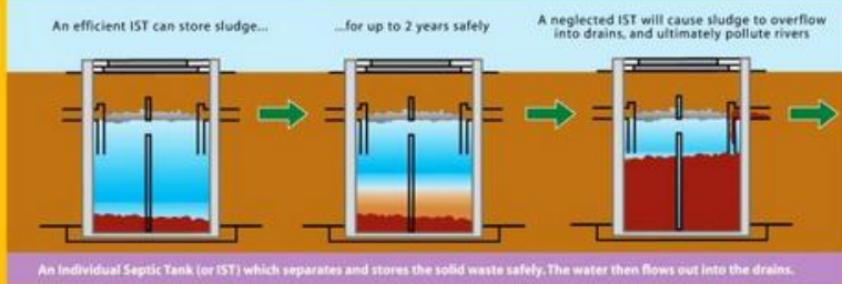
An Individual Septic Tank (or IST) which separates and stores the solid waste safely. The water then flows out into the drains.
