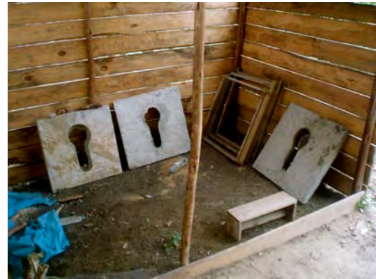
Local workshop producing SanPlat latrines in the Commune of Andasibe
