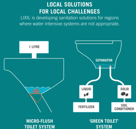
**The Micro-Flush Toilet System improves the water efficiency of toilet and sewage systems.**
